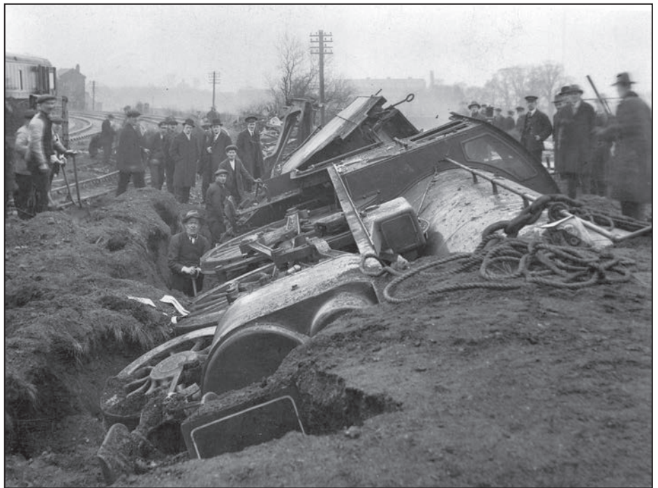
LNER D49 4-4-0 No. 2758 Northumberland lies on one side deeply embedded after a high speed derailment on the curve between Willowholme Junction and Port Carlisle Branch Junction. 3rd January 1931. CRA Peter W. Robinson Collection PWR-V0028.
