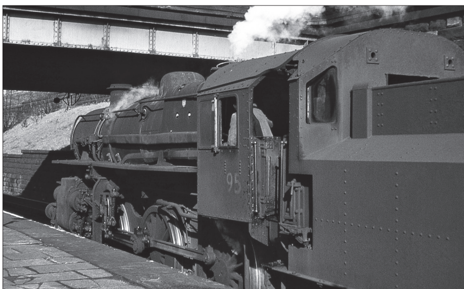
LMS 4MT 2-6-0 43095 in Platform 5 on Lancaster Castle station with the M&GN tablet catcher clearly displayed. 3rd March 1966. Ron Herbert.
