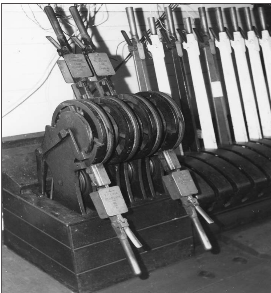
When Lindal East and Lindal West were amalgamated into a new box at Lindal Ore sidings on 26th November 1939 the entrance to the Down loop and exit from the Up loops were too far away for conventional point rodding. A continental system of wire operated points was used instead. Here the barrel type levers are shown. Motor points replaced these wires shortly before the box closed in 1978. They had a reputation amongst older signalmen of being difficult levers to operate.
